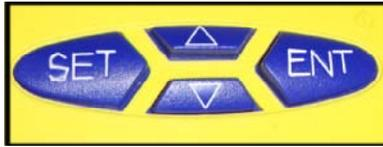
**PRESS and hold ENT for 1 SECOND,**.....”ENT” key to “**POWER ON**” the terminal.
